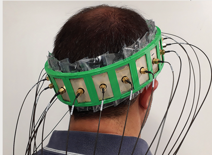
A new smart helmet uses electromagnetic waves to estimate the size and position of a stroke inside a patient’s brain.
